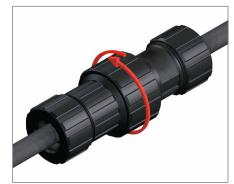
Lock the Central Locking Ring using the remote locking / release key.
