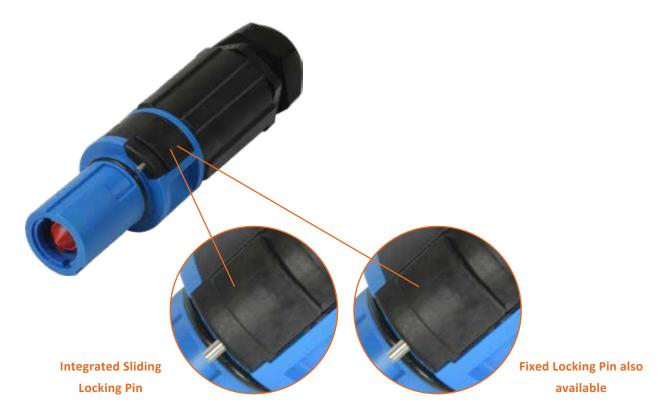
Most versions of this connector format have relied upon the electrical contact being retained within the insulator by means of a plastic dowel/cotter pin. These pins are forced through a mating hole in the Insulator and contact and any re-use of the same pin may adversely affect the IP sealing of the connectors.
